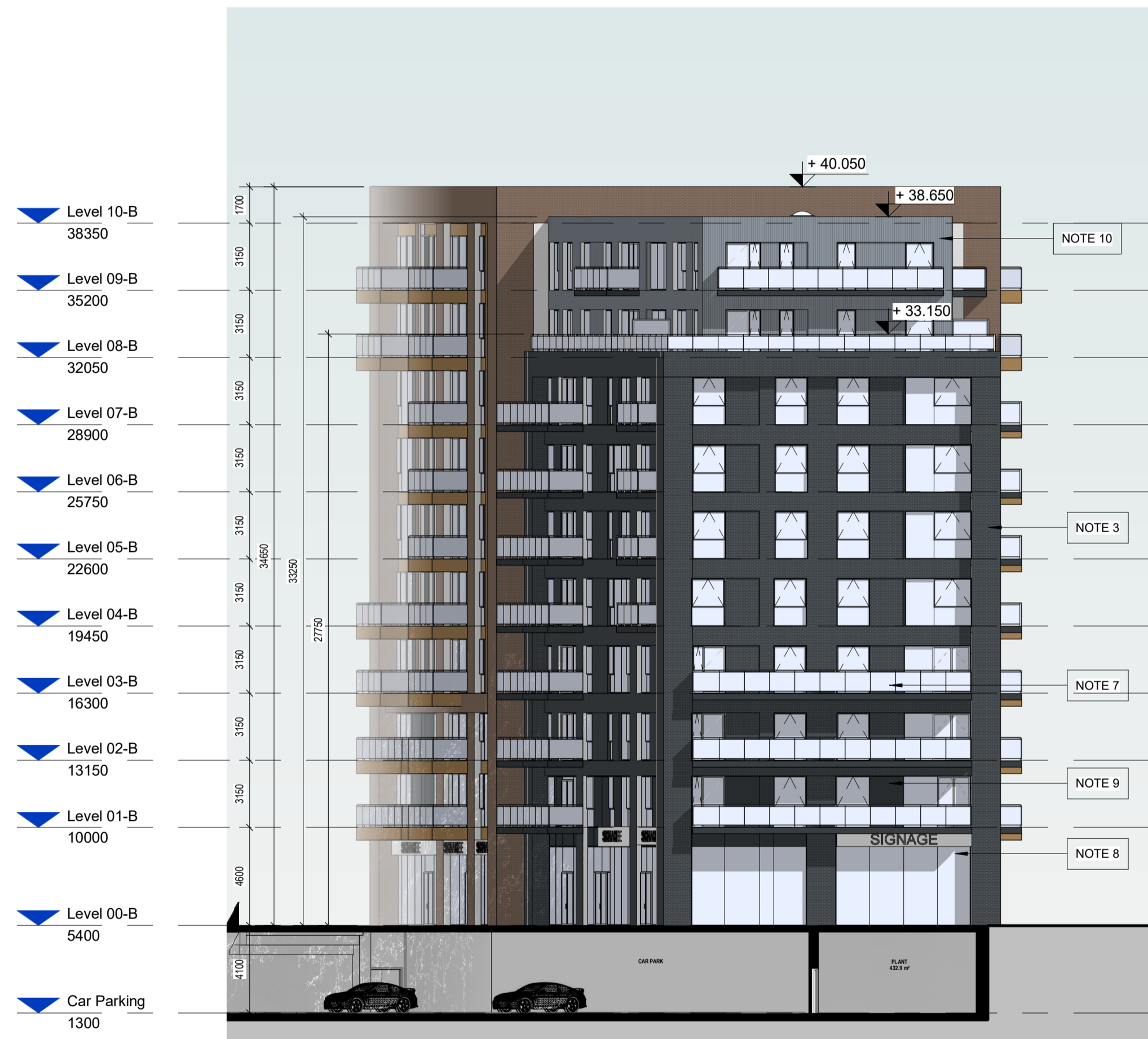
1 BLOCK B-EAST ELEVATION 1 : 200
