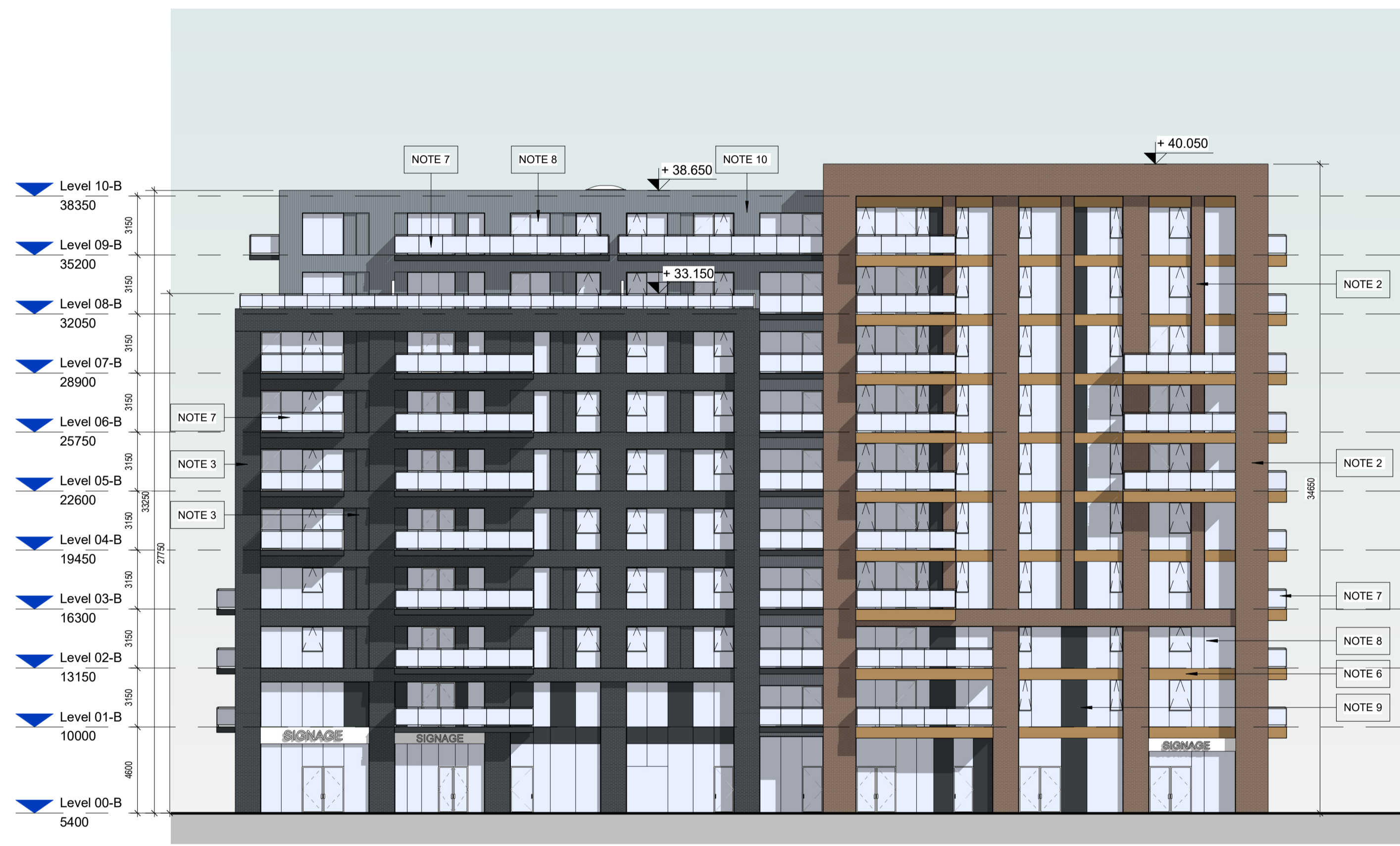
2 BLOCK B-NORTH ELEVATION 1 : 200
